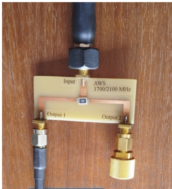
Fig. 14. Power divider with load resistor at output 2
